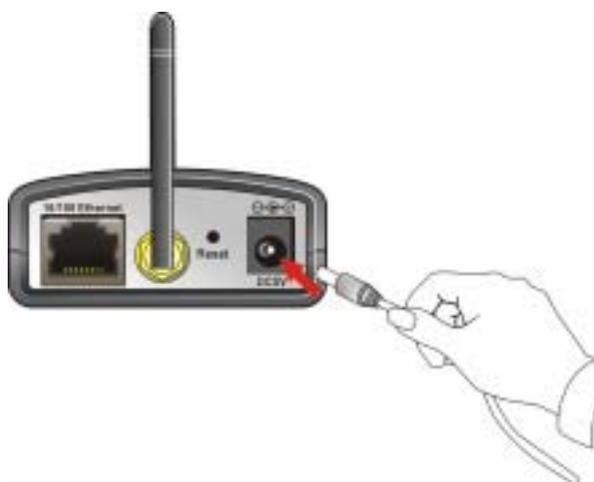
**TIP:** You can confirm power source is supplied from the LED indicators label Power on the Wireless Internet Camera is illuminated.
