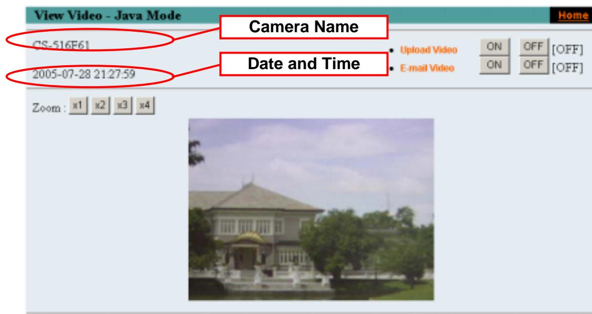
**Camera Name:** The Camera name will be displayed when the Camera Name field is entered in the Web Configuration setting under **Configuration**.
