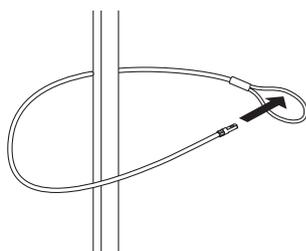
1. Loop the cable around a secure object.
