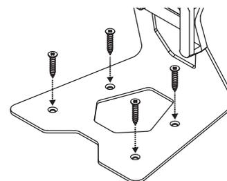
Use the screws included to fix the stand on wooden surface.
