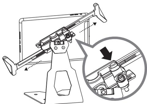
1. Press and hold on the release button to unlock the frame.
