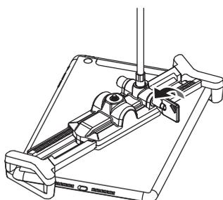
1. Insert the key into the lock button to release the cable.
