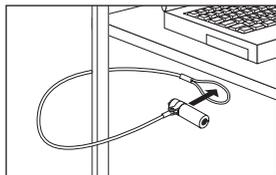
Loop the cable around a secure object.
