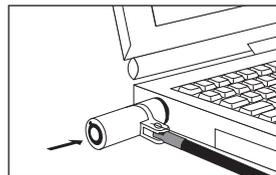
Press the button to lock the security cable.
