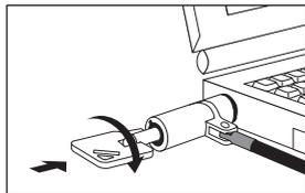
Insert the key and turn it clockwise to unlock the cable.
