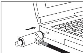
Insert the lock into the security slot of the computer.
