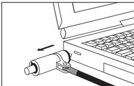
Remove the cable from computer's security slot.
