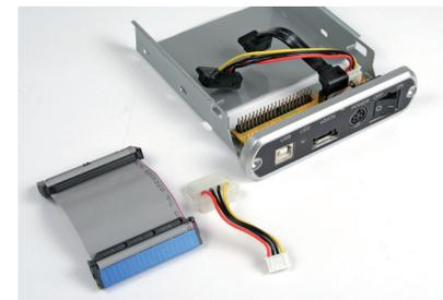
4. In case of SATA Hard Drive, replace the IDE cables with the SATA ones enclosed in the package.
