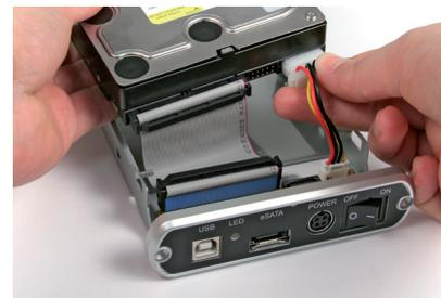
3. Connect the 44-pin IDE connector and the power connector from the base plate securely to the Hard Drive.
