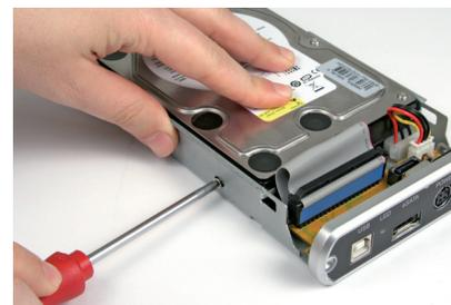
5. Place the Hard Drive in the base plate and fix it with the 4 screws.
