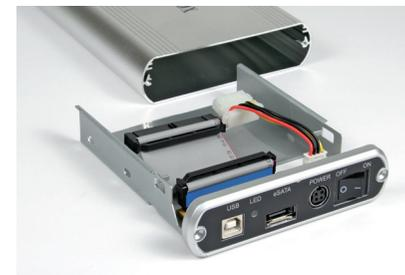
2. Draw the back panel/base plate out of the aluminum enclosure.
