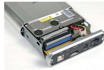
5. Slide and push the HD/Base Plate into the aluminum enclosure, then fix the back panel with the screws. The enclosure is now ready to use.
